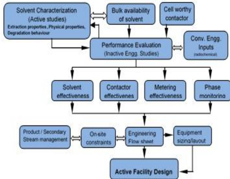
**Fig. 4: Overall R&D Programme for Partitioning of HLW**
