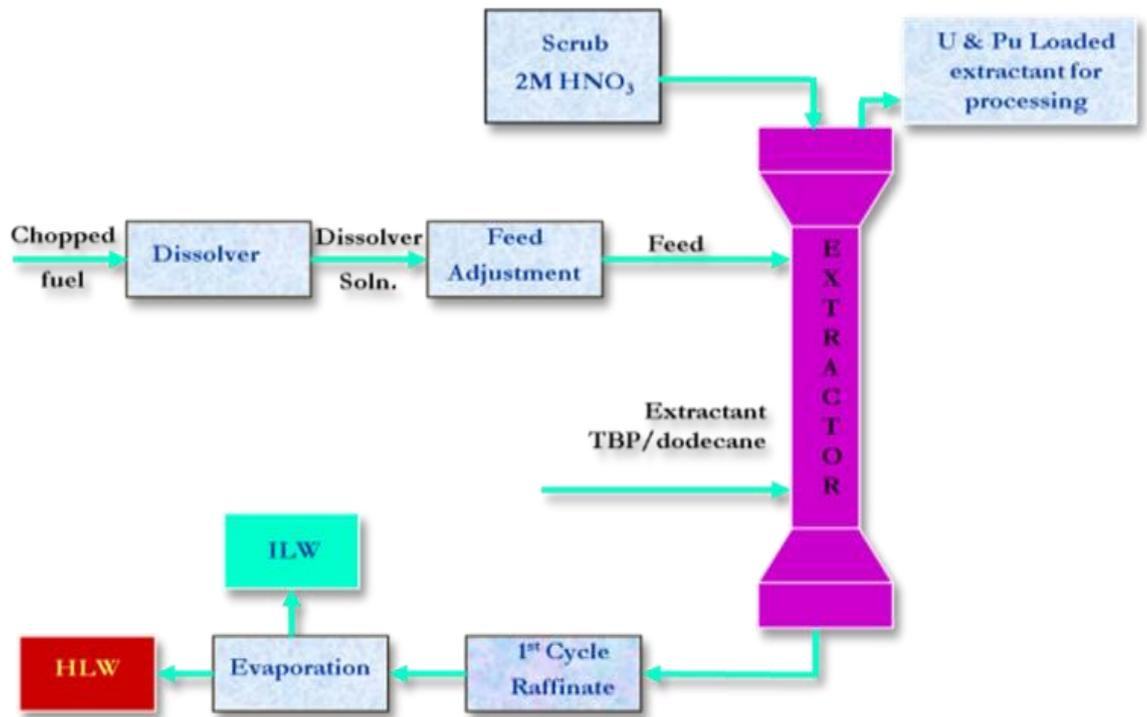
**Fig. 1: Generation of HLLW from reprocessing of spent fuel**
