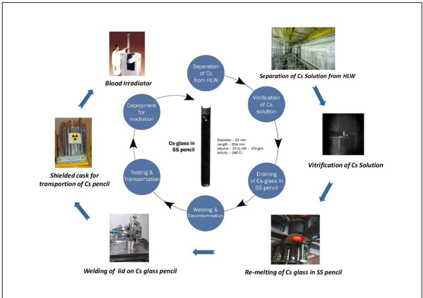
**Fig. 2: Cs glass pencil production process**
